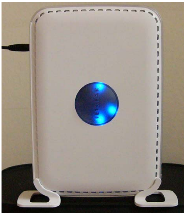
Figure 4-1: Vertical orientation required on metallic surfaces
